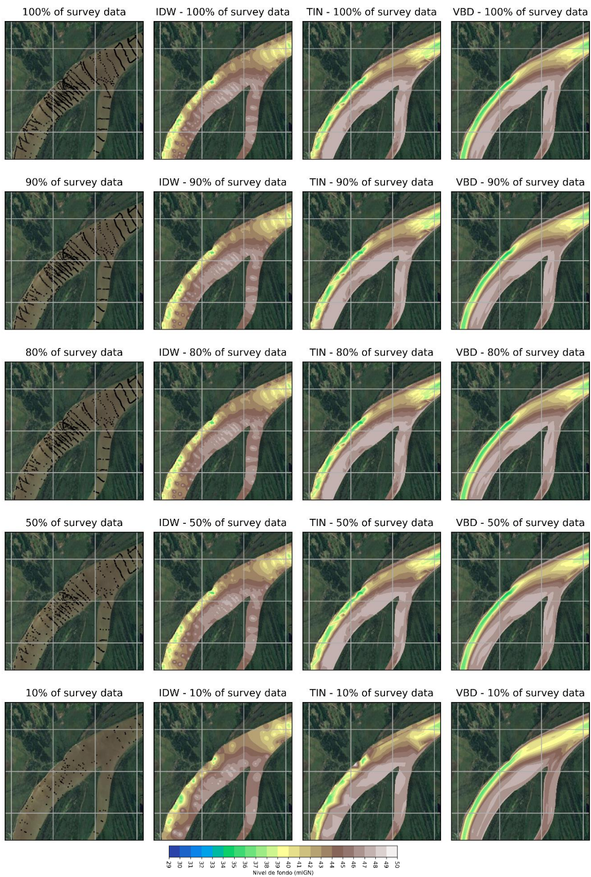
Figure 5: Comparison of the performance of IDW, TIN and VBD methods with different decimations of the source dataset.
